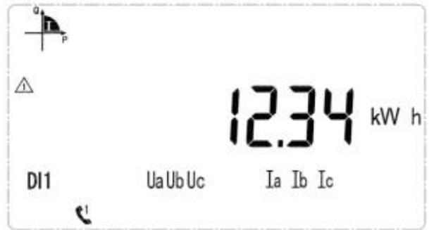
Current forward active spike energy 12.34kWh
