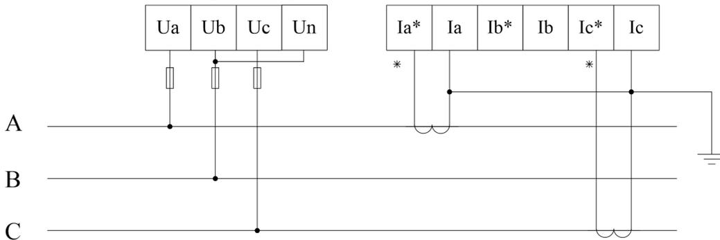
Fig 5 Three phase three lines connect via CT
