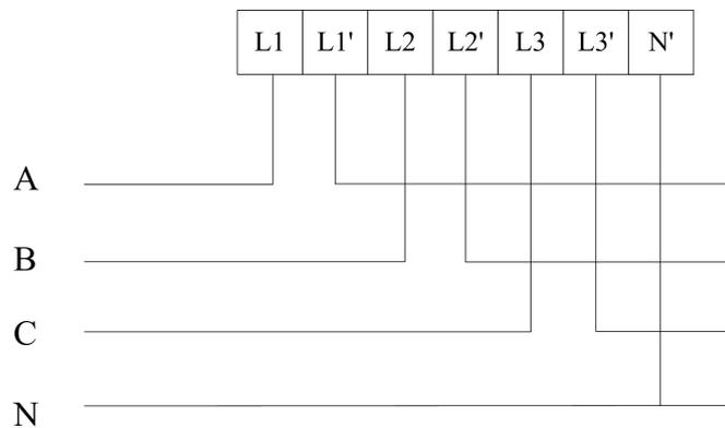
Fig 4 Three phase four lines direct connect
