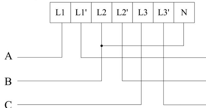
Fig 6 Three phase three lines direct connect
