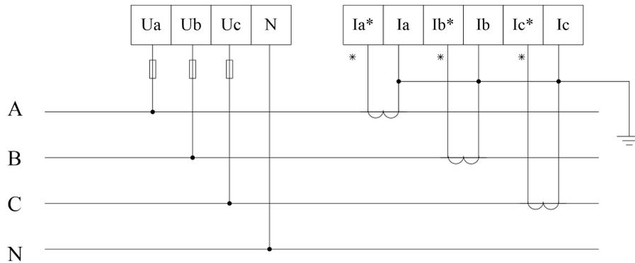
Fig 3 Three phase four lines connect via CT
