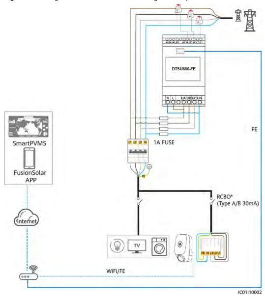
Figure 3-2 Charger connected to a router through the FE port or WiFi
