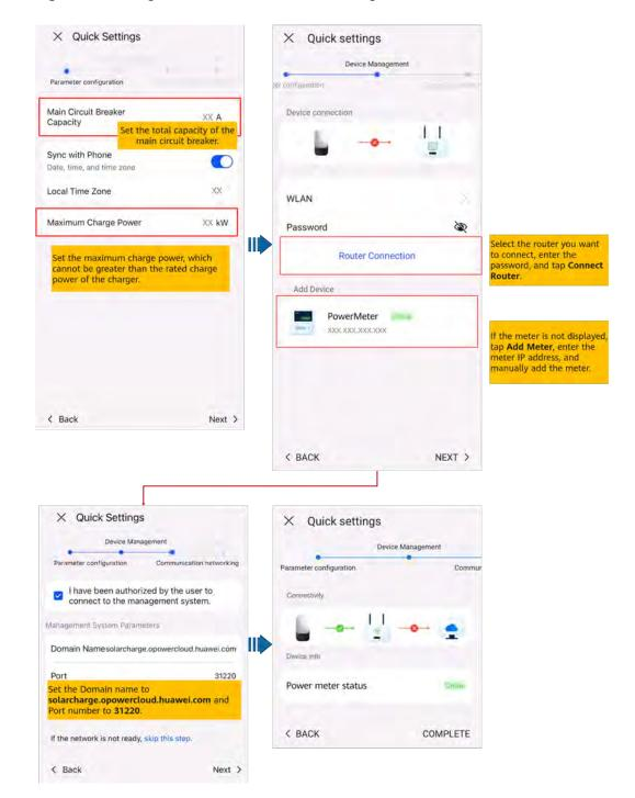
Figure 4-8 Charger connected to a router through WiFi
