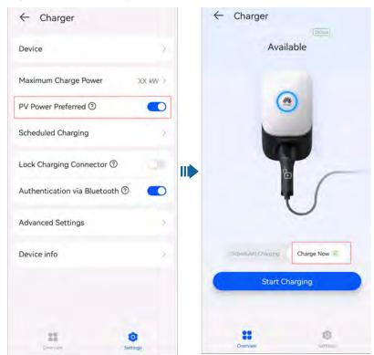
Figure 2-10 Enabling PV power preferred
