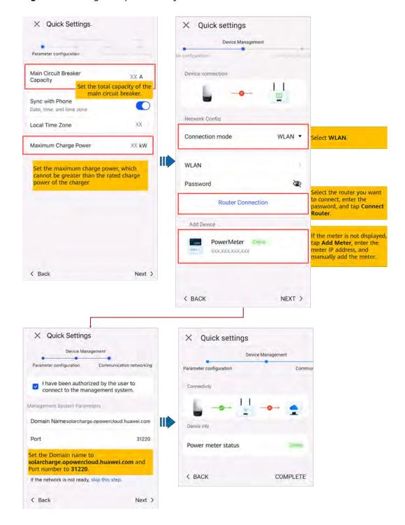
Figure 4-6 Charger FE port directly connected to a meter
