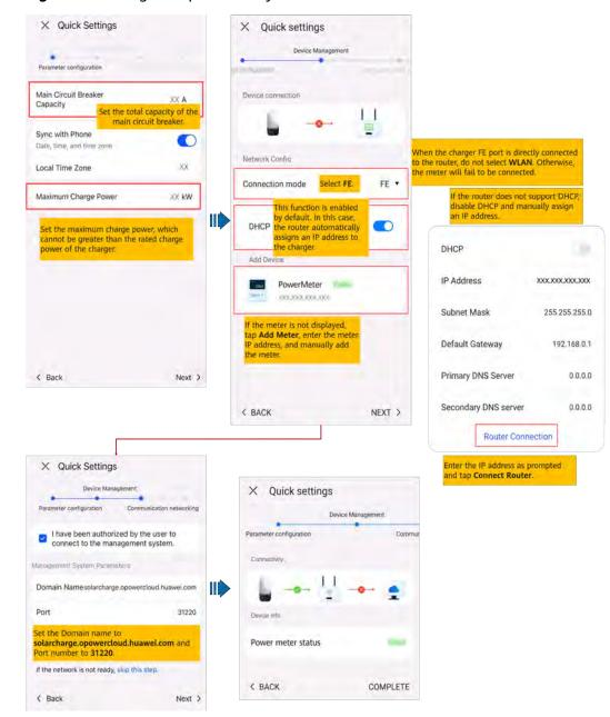
Figure 4-7 Charger FE port directly connected to a router
