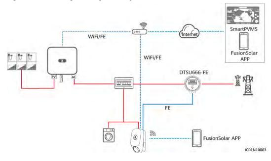
Figure 2-4 PV+Charger (charger directly connected to a FE meter)
