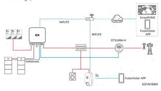
**Figure 2-5** PV+Charger/PV+ESS+Charger (RS485 meter & FE meter & WLAN/FE Smart Dongle)
