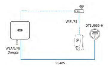
Based on meter connection modes and PV device configuration, the installation scenarios are classified into Charger-only, PV+Charger (FE meter), PV+Charger/PV+ESS+Charger (RS485 meter & WLAN/FE Smart Dongle), and PV+Charger/PV+ESS+Charger (RS485 meter & FE meter & non-WLAN/FE Smart Dongle).
