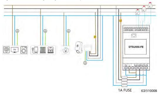
Figure 3-6 Connecting charger L1 to the phase wire with the minimum load
