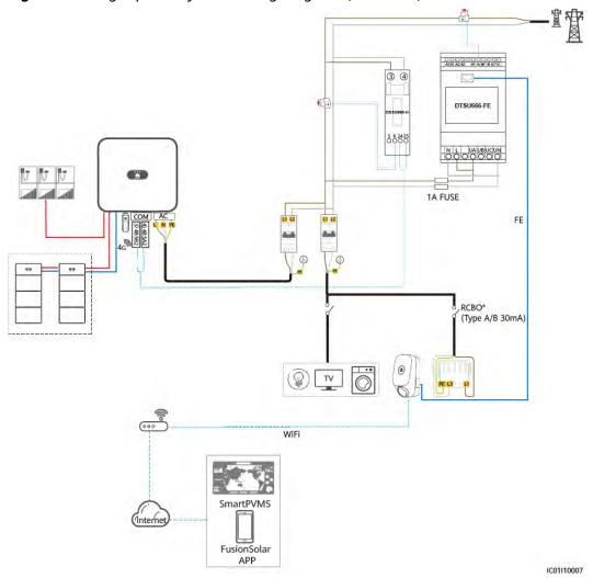
Figure 3-8 Single-phase system wiring diagram (230 V L-L)
