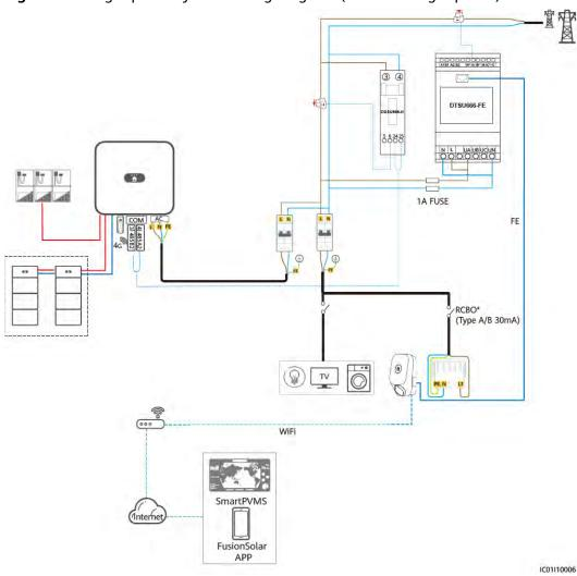
Figure 3-7 Single-phase system wiring diagram (TN & TT single-phase)
