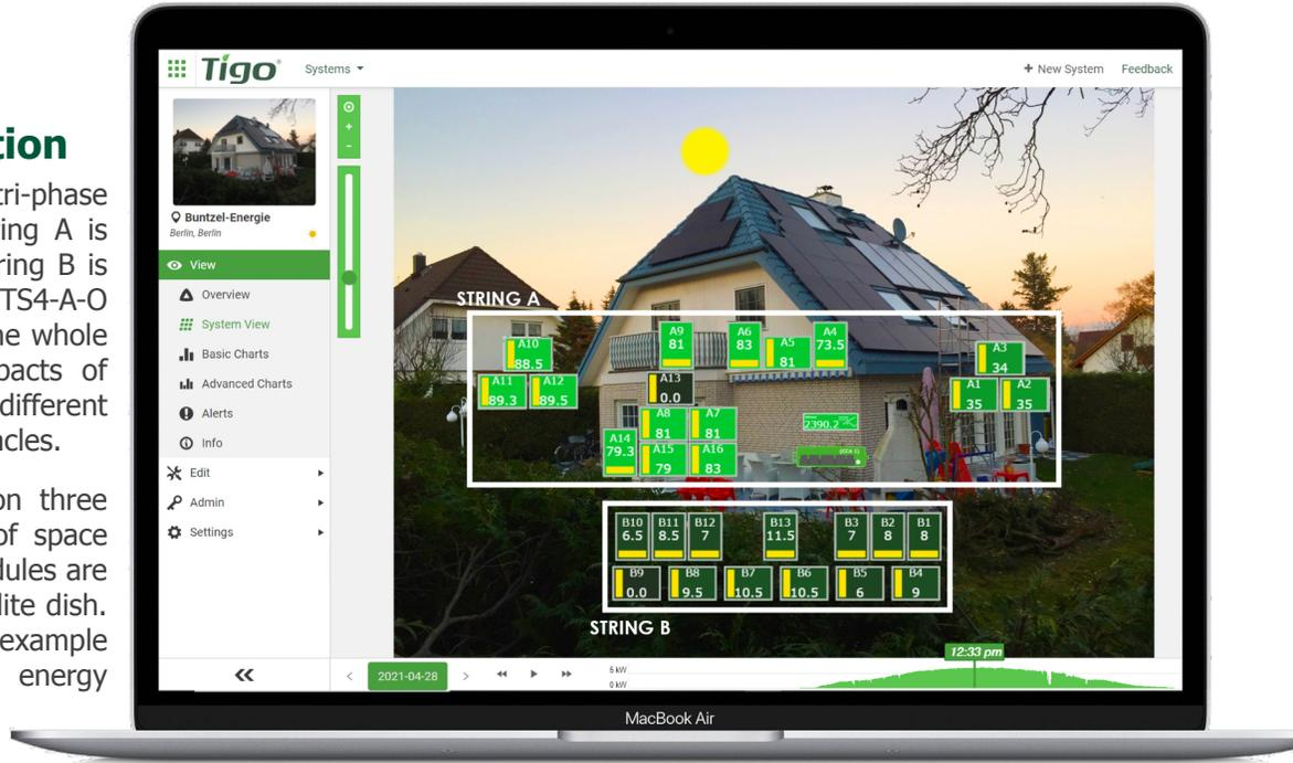
Without optimization, the inverter would choose a lower operating point for the string and the unshaded modules would contribute less than what they can produce under the site conditions. Instead, the best performing modules stay at the maximum power point set by the inverter and the optimizers adjust their output for the best result.
