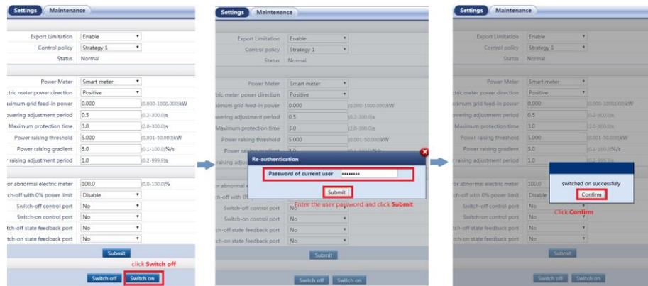
After switch-on is complete, check whether the circuit breaker is ON.
