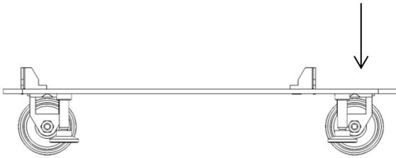
First place, the ground plate to the place where the Power Battery to stand later. Keep a distance of 20cm away from the wall.
