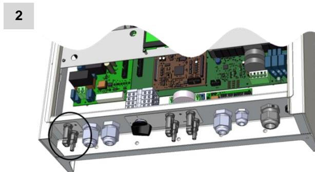
Connect the DC cable into the Power Battery Master.
