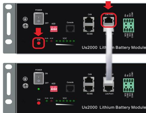
(3) Press the **red button** of **master battery** to power on, all the battery LED light will be on one by one from the Master battery:
