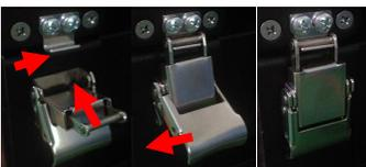
Aim at the 4 pare of Location Pin and Location Hole, stack the batteries together. And hasp the 4 agraffes together.
