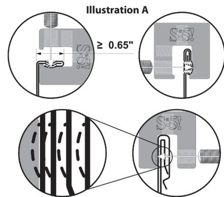
(Top) S-5-U clamp on both vertical and horizontal seams. (Bottom) S-5-S on a snap together seam with blow up illustrating deformation of seam as setscrew is tightened. **For horizontal seams equal to or greater than .65" use the S-5-U in its horizontal orientation.** **For horizontal seams equal to or less than .50" use the S-5-S mounted vertically.**
