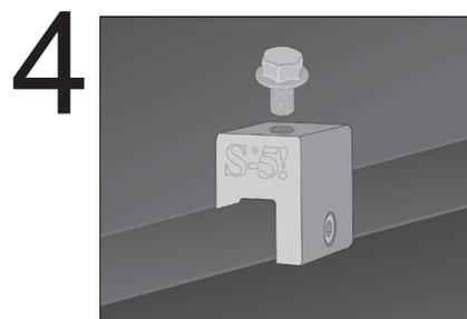
Above illustrations show S-5-E Mini clamp on a vertical seam. Step 2 shows S-5-E Mini on vertical applications and S-5-U Mini on horizontal applications.
